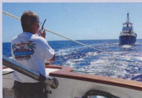
Atlantic Escort pumps fuel to Uno Mas through a simple garden hose while crossing the Atlantic.
